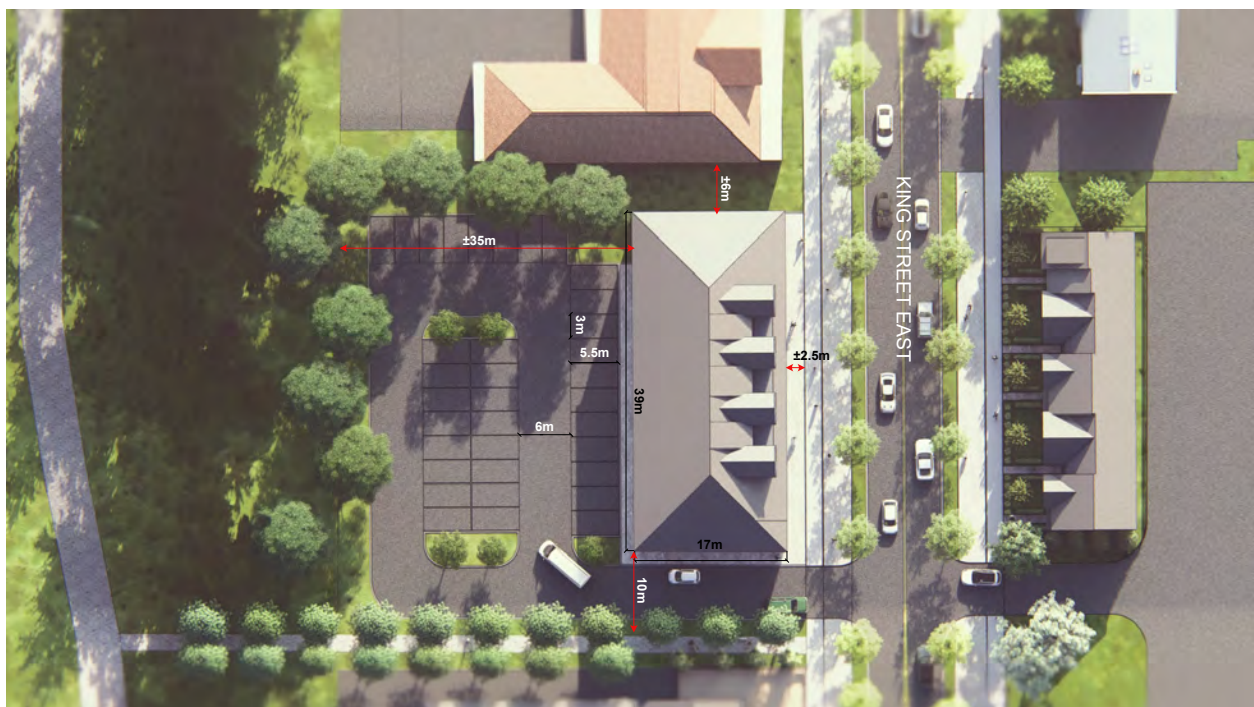
Conceptual Four-Storey Building Site Plan
